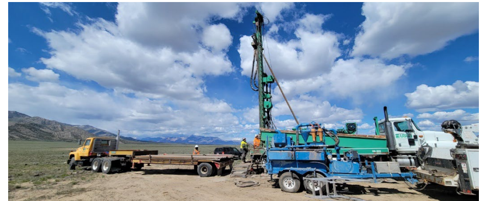
Borehole Cleaning and P-S Suspension Testing Activities
