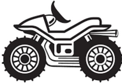
**Off-Road Vehicles (ORVs)**, also known as **Off-Highway Vehicles (OHVs)** are a class of motor vehicle designed for use over unimproved terrain, and include all registered motor vehicles if used for recreation off a public way. This class of motor vehicles includes **All-Terrain Vehicles (ATVs)**. **Vehicles exceeding 1,000 lbs.**, such as pickup trucks and SUVs, are not considered ORVs and **are prohibited from trails at all times.**
